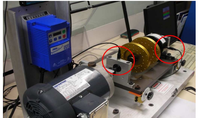
Fig. 3. Experimental setup. The sensors are placed in the red circles respectively.
