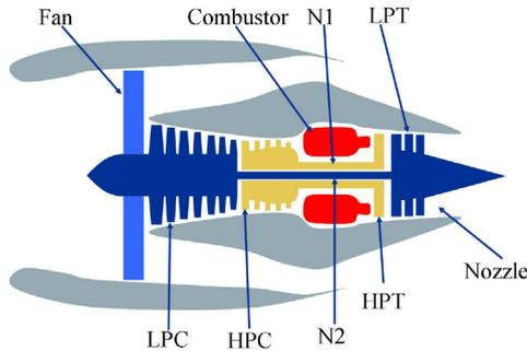
Fig. 5. Diagram of the engines in C-MAPSS data [27].
