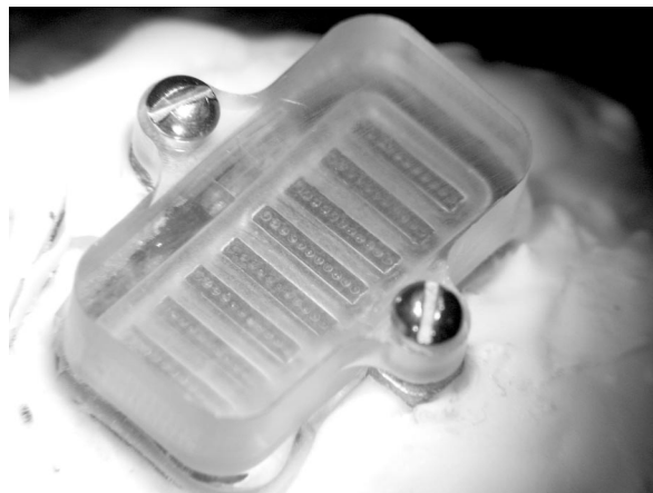
FIG. 3. Single-row connector bank; dual-row assemblies were also made. The housing was machined from polycarbonate with grooves to hold 10-pin, 0.025\text{-in} center Omnetics connectors, sealed in with epoxy. A polycarbonate cover was secured with screws, with an O-ring in between to make a water resistant seal. The Omnetics connectors are visible through the cover. The epoxy around the connectors prevented moisture from seeping up from underneath. The connector assembly is shown mounted to the acrylic skull cap.
