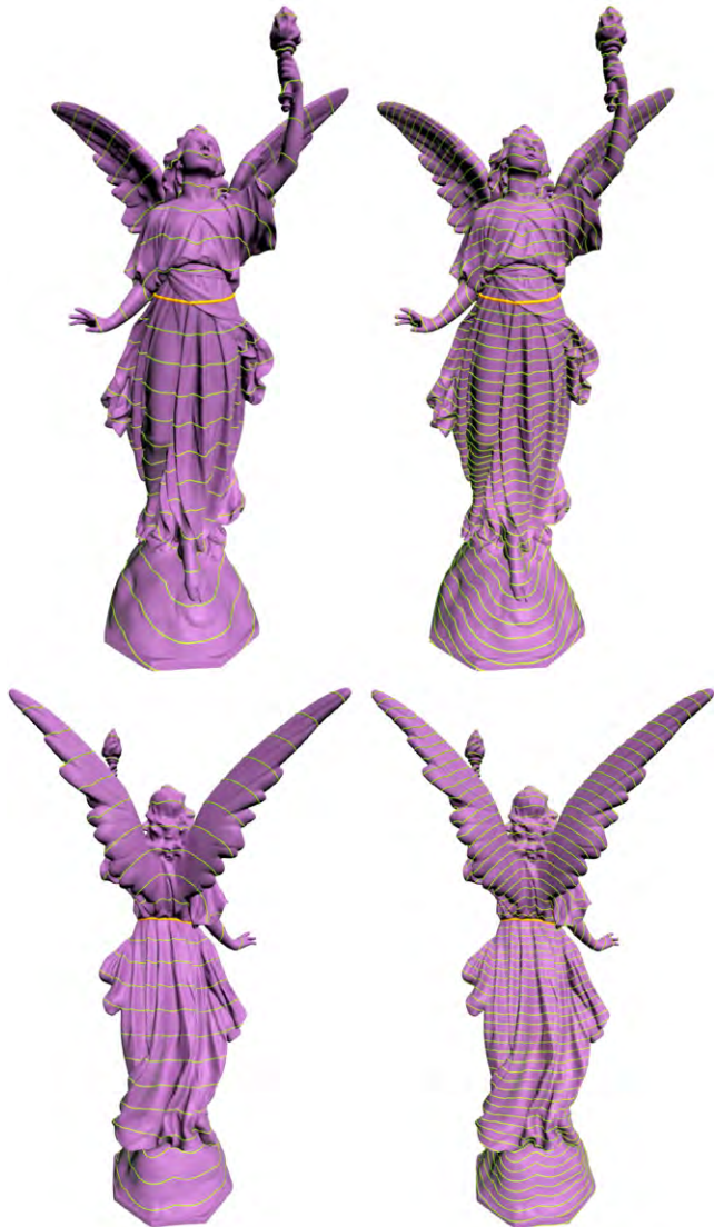
Fig. 11. Given the generator curve on the waist, we compute the geodesic distance field of the Lucy model. Here we show the set of offset curves with spacing of 0.06 (left) and 0.025 (right) respectively. The model is normalized to a unit cube.
