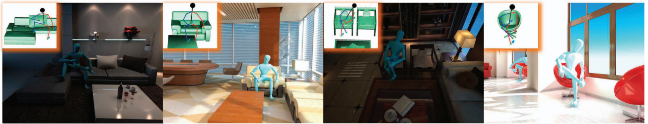
Fig. 1. Various sitting poses designed by our system. The user sketches the 2D stick figures on the screen space to specify the desired poses in a virtual environment (see the inset of each subfigure), and our system automatically generates the physically correct and visually pleasing 3D poses at interactive speed.
