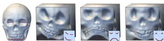
Fig. 4. The users can take full control of the polycube map by simple sketches. The thumbnails show the sketched constraints.
