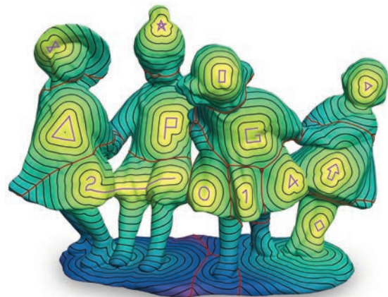
Figure 1: The polyline-sourced geodesic Voronoi diagram (GVD) on triangle meshes. The generators, bisectors and iso-distance contours are drawn in pink, red and black, respectively. The color indicates the distance to the generators.
