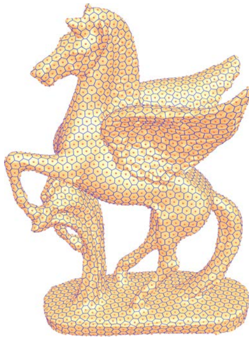
Figure 1. Our intrinsic method can compute a high-quality centroidal Voronoi tessellation on model with complicated geometry and topology. The CVT on the Pegasus model was created by 3000 sites.
