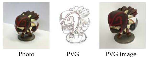
Fig. 24. PVG is able to produce photo-realistic images with sparse geometric primitives. This PVG consists of 85 diffusion curves (solid lines), 71 Poisson curves (dashed lines) and 24 Poisson regions (loops with hatches).
