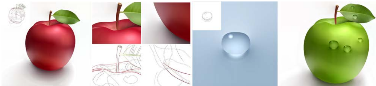
Fig. 1. A Poisson vector graphics (PVG) consists of the popular diffusion curves (DCs), specifying the boundary colors, and two new types of primitives, called Poisson curves (PCs) and Poisson regions (PRs), which are associated with Laplacian of colors. The key idea of PVG is to explicitly separate colors and tones so that editing hue and tone is easy and intuitive. For example, we can make a green apple by simply changing only the DCs' color from red to green. Note that all the PCs and PRs remain unchanged. PVG natively supports seamless cloning: The water droplet can be directly copied to the target and then it automatically fits into the new background. DCs, PCs and PRs are depicted by solid lines, dashed lines and loops with hatches, respectively.
