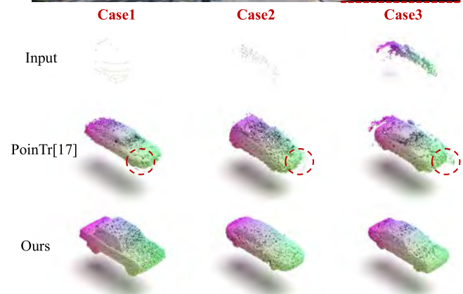
Fig. 7. Qualitative point cloud results on the KITTI (car) dataset by different methods. We compare our method with the approach of PoinTr across three varying cases of completion difficulty. Best viewed in colors.
