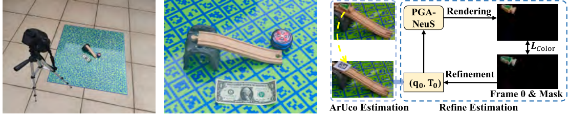
Fig. 3. Data acquisition. Left and middle: We use a single camera to capture dynamic scenes involving moving rigid objects in a static environment. As the camera is mounted on a tripod and positioned to shoot the scene from a high angle, given that the objects are relatively small (typically less than 10 cm), some regions may be obscured due to occlusion and self-occlusion. Right: Estimating the initial pose involves using an ArUco marker to determine the object’s rough position and orientation. Then, PGA-NeuS refines this estimate by minimizing the color loss between the rendered image and the masked first frame of the input video.
