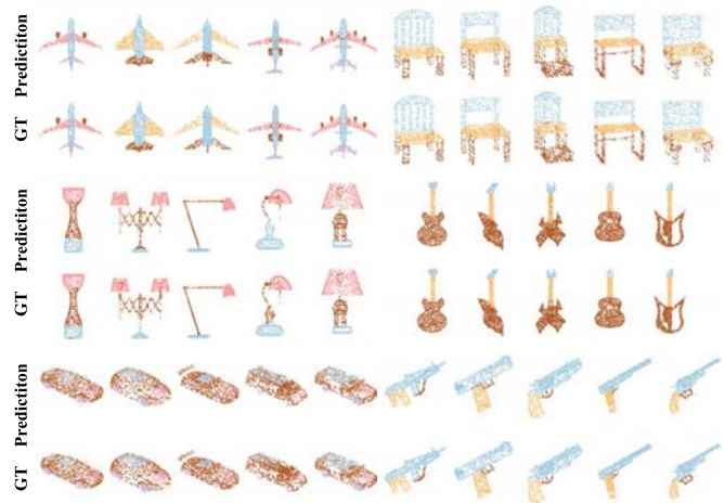
Fig. 4. Visualization of part segmentation results. Different colors can be ascribed to different parts of the objects. The top row depicts results predicted by Curriculumformer, while the bottom row shows the ground truth.
