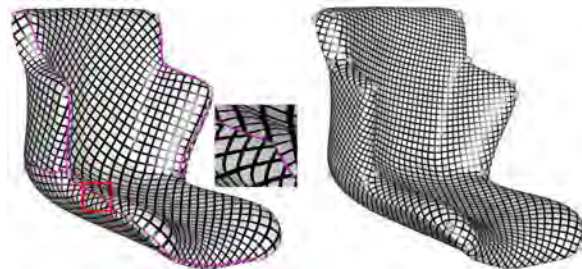
Fig. 21. Our method can be extended to compute smooth N -RoSy fields for various values of N . Illustrated here is a 6-RoS field applied to a two-holed torus, featuring 16 valence-7 and 6 valence-5 vertices, while all other vertices maintain regular valence of 6.
