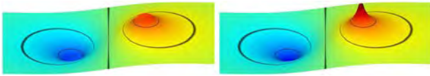
Fig. 8. This illustration compares two sets of singularities with identical indices but varying radii. The singularities on the left feature larger radii compared to those on the right. The set with smaller radii generates a more intense vector field, \nabla\varphi , characterized by steeper peaks and deeper valleys in the value of \varphi . We depict \varphi using a color-coded height function to visually represent these variations.
