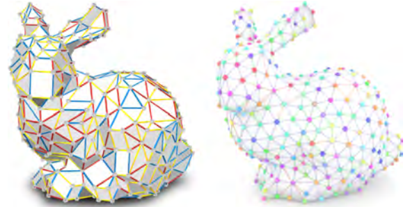
Fig. 18. Comparing (left) Zometool shape approximation [4] with (right) our approach. Our approach is able to better approximate the BUNNY model using a smaller number of vertex classes and a smaller number of edge classes; see Table III for the statistics.
